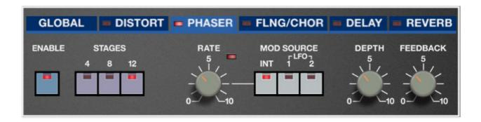
**Enable**- Enables and disables phaser effect. The LED in the tab additionally indicates current enabled or disabled status.
