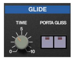
Glide delays the voltage change between notes for a sliding pitch effect.
