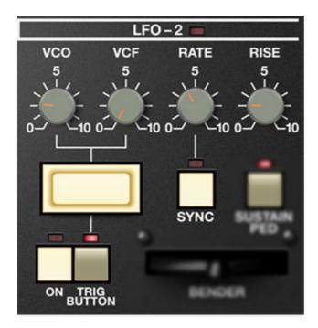
On the original instrument, LFO-2 was "performance only," that is, the only way to activate it was to press (and hold) the big button. We've increased LFO-2's usefulness by allowing user selection of standard trigger button activation or always-on mode.
