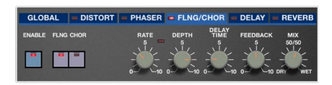
We've included a thick and warm flanger/chorus effect. Flanging and Chorus are closely related - the general difference being that flangers use a shorter time range and some amount of feedback (this intensifies the "jet-flyby" whoosh), whereas choruses utilize a slightly longer delay time, and no feedback.
