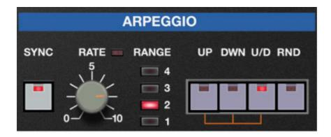
An arpeggiator is basically a step sequencer that plays each note of a chord individually in an ascending or descending pattern across one or more octaves.
