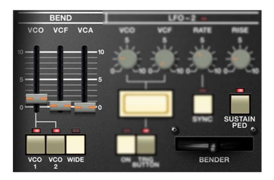
The original instrument had a joystick bender control that moved on a horizontal axis, plus large on/off button for initiating modulation. Roland made up for the lack of a variable mod control with a clever joystick implementation that allowed the joystick to control VCO pitch, VCF cutoff, and VCA volume.
